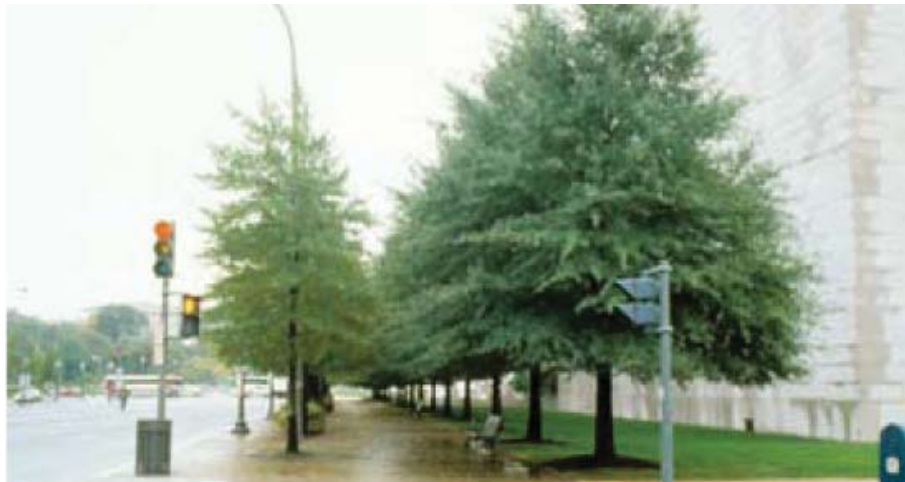
Fig #48 Trees planted at the same time, but with different soil volumes
